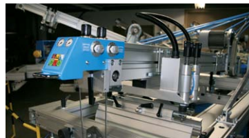
Swivelling printing arm for easy access and better setting of the screen
